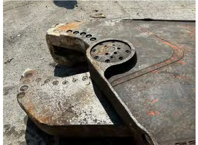
A hydraulic steel shear lays in wait for use on Phase II. The shear cuts steel I-beams into manageable sizes for recycling.
