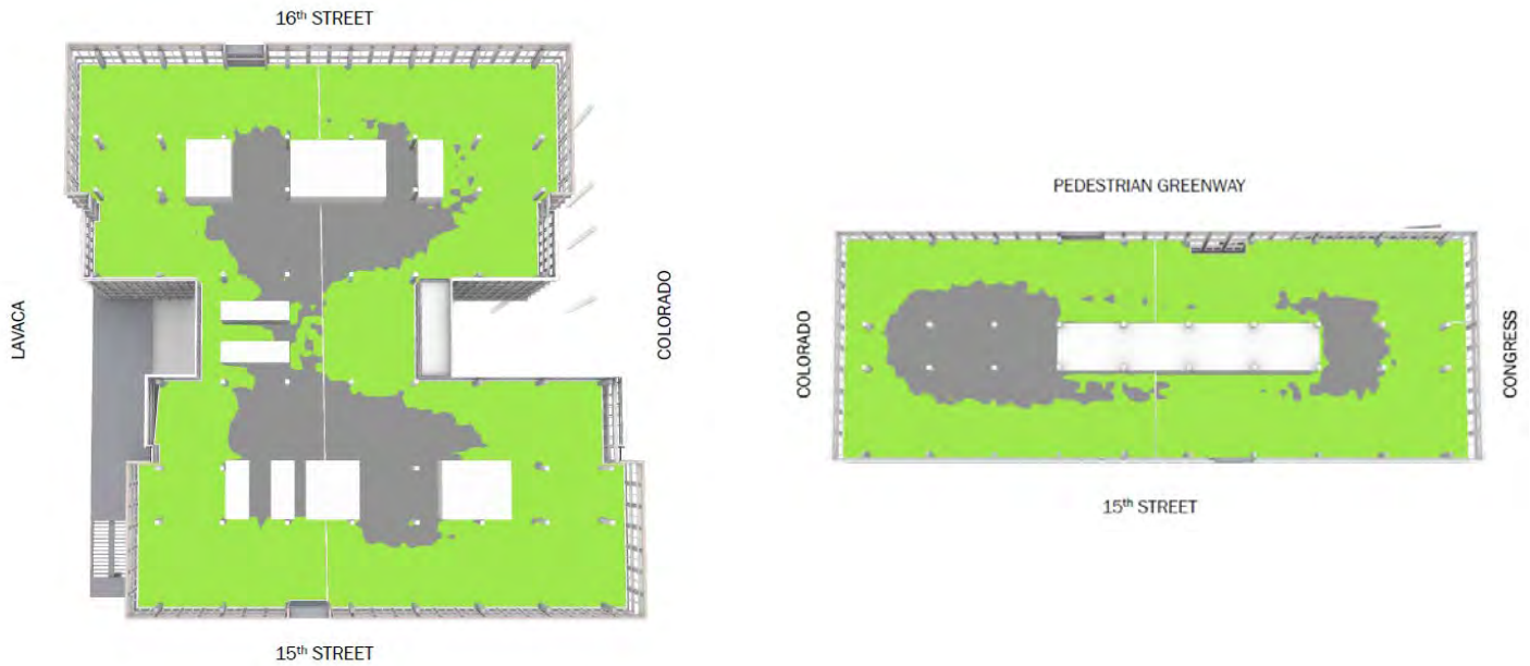
Daylighting modeling for 1501 Lavaca and 1500 Congress State office buildings. The green area depicts the interior areas that will receive natural light.
